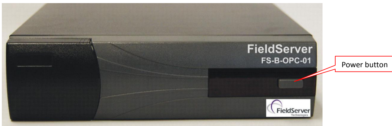
Figure 4-1: View of front of FS-B-OPC-01 Showing Power LED and power button
